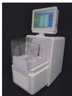
Protein detection system using a personal protein chip
